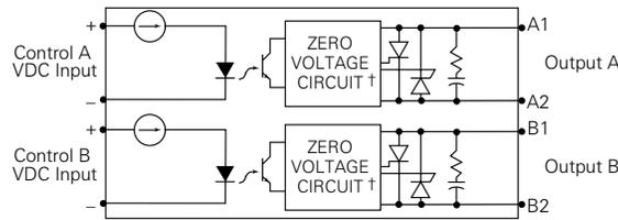
† Random Turn-on Units have a Random Turn-on circuit instead of Zero Voltage Circuit
